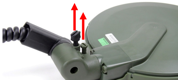
Figure 56: Removing two (2) Screws
