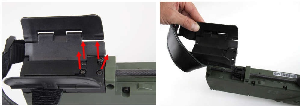
Figure 9: Removing the Armrest
