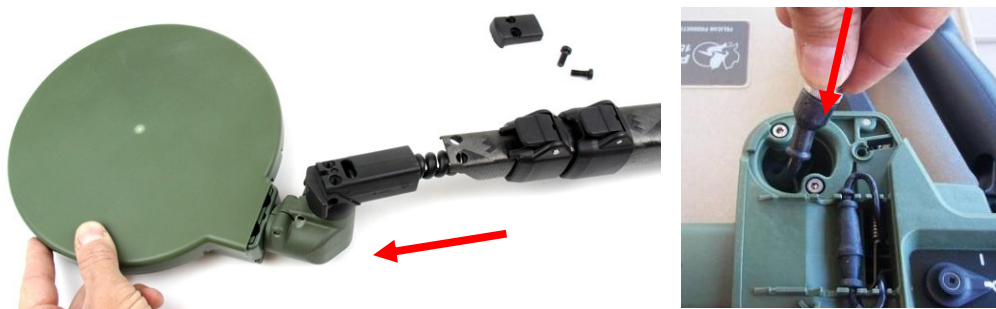
Figure 53: Sliding the Coil Off the Shaft
