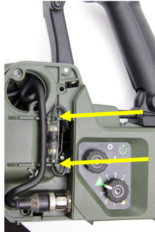
Figure 85: Correct Position of Wiring Loom Handle
