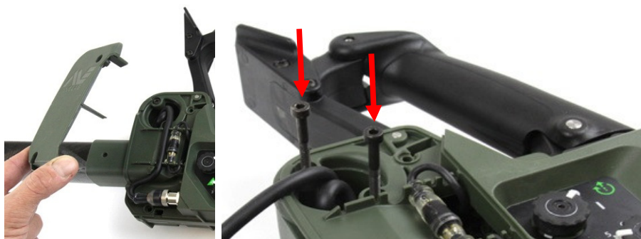
Figure 25: Fitting Screws into the Shaft Hinge
