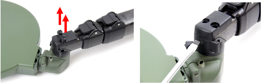
Figure 52: Removing Screws from Lower Shaft
