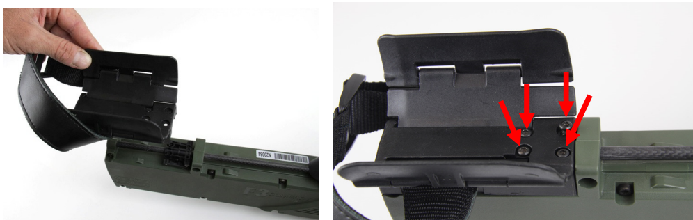
Figure 28: Attaching the Armrest
