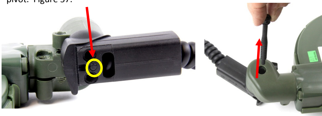
Figure 57: Removing Pin Coil Pivot
