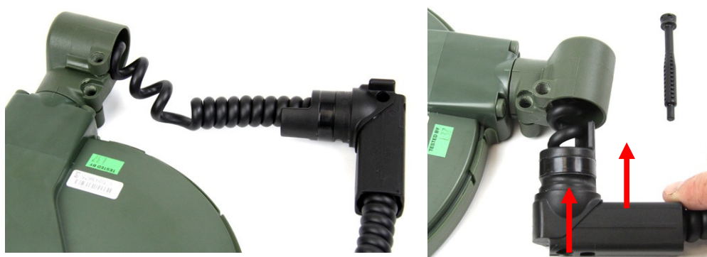
Figure 62: Fitting Pivot Lower Shaft
