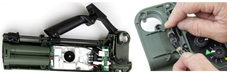
Figure 80: Disconnect Wiring Loom Handle
