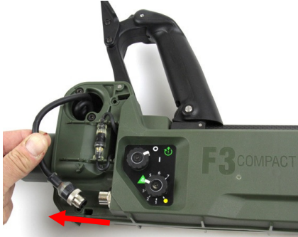
Figure 50: Disconnecting Coil Connector
