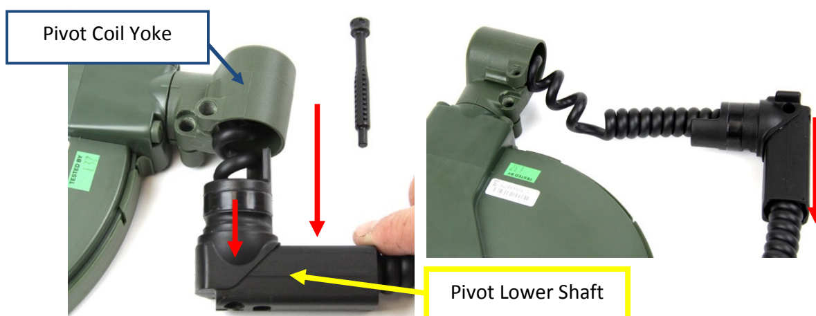
Figure 58: Removing Pivot Lower Shaft
