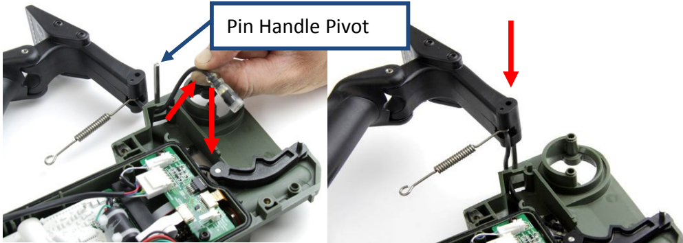
Figure 83: Threading the Wiring Loom
