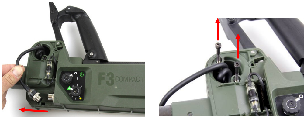
Figure 11: Disconnecting Coil Plug and Removing Screws
