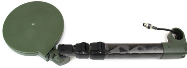
Figure 74: Shaft and Coil Removed from Detector
