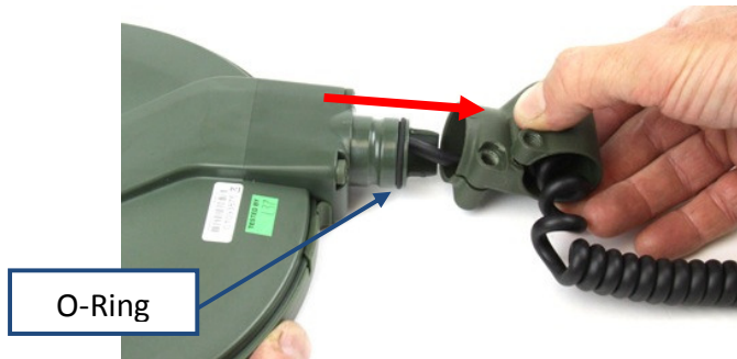
Figure 59: Removing Pivot Coil Yoke
