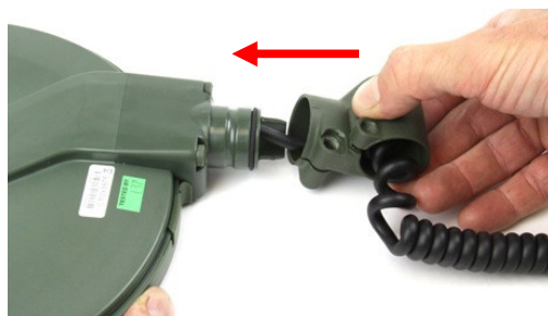
Figure 61: Fitting Pivot Coil Yoke
