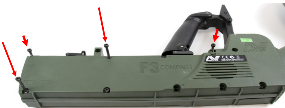
Figure 23: Fitting Four Screws
