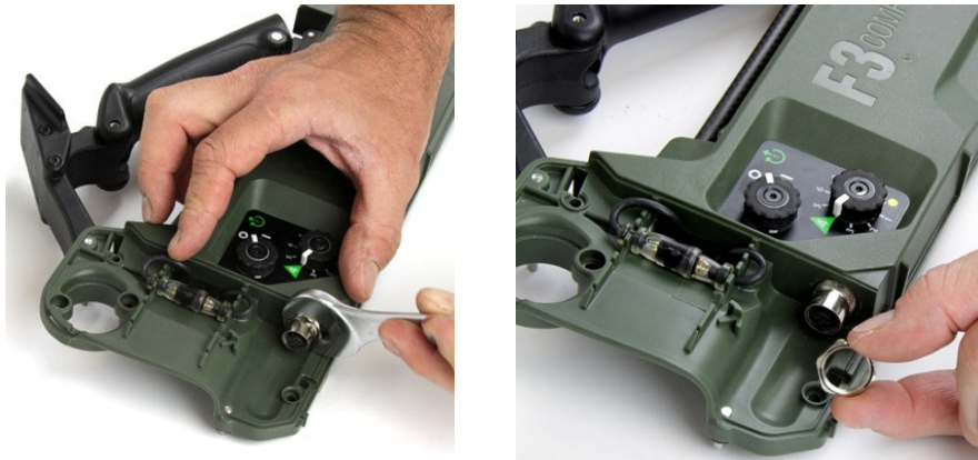
Figure 32: Removing the Coil Connector Nut (18mm)
